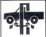
Use height extenders when necessary to ensure good contact.
