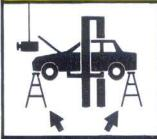
Always use safety stands when removing or installing heavy components. · ©
