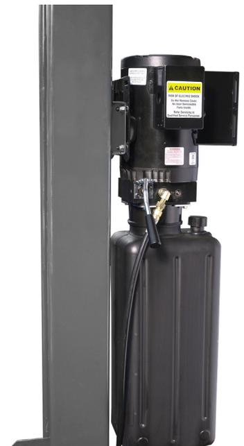
An air supply (minimum 30 psi / 3 CFM) is required for the safety-lock mechanisms to disengage. It is solely the responsibility of the end-user to provide, install and maintain the air supply.
