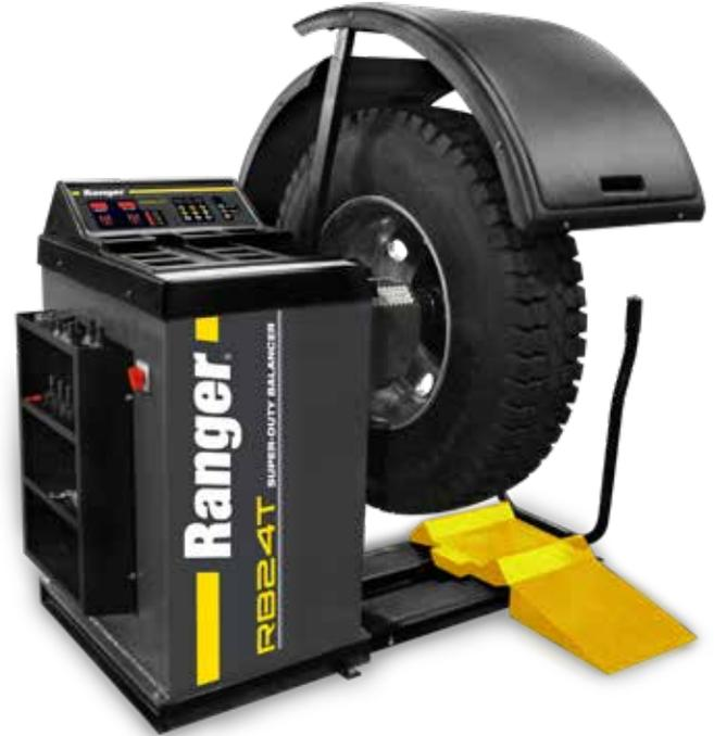
The RB24T truck wheel balancer handles tires up to 50" in diameter, 20" wide and rim sizes up to 30" in diameter. Although best suited for bus, truck and OTR wheels, it's capable and fully equipped to accommodate automobiles and light truck wheels as well. An integrated wheel lift easily lifts the heaviest wheel assemblies for effortless mounting on the balancer.
