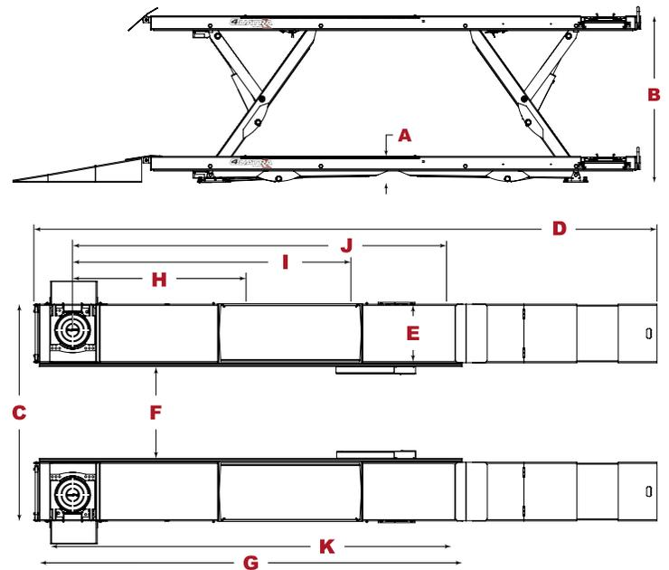
Note: An air supply (minimum: 30 psi / 3 CFM) is required for the safety-lock mechanisms to disengage. It is solely the responsibility of the end-user to provide, install and maintain the air supply.
